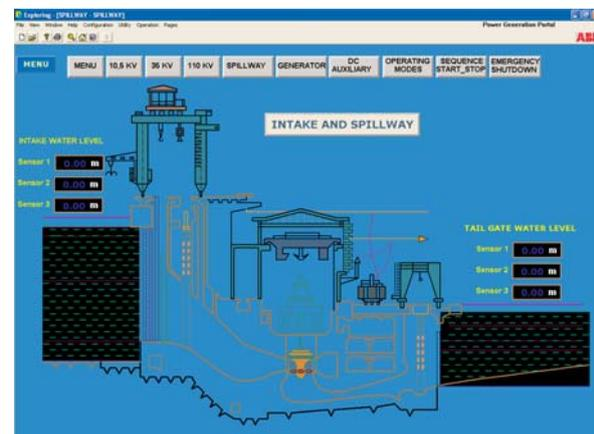
Fig. 3: Spillway control of a hydro power plant
